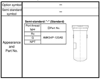
Note1) Part No.③ includes Bowl seal ②. Refer to [10. Disassembly Drawing ](P15).
