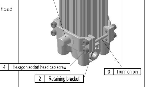
\* When it is difficult to place the head cover side facing downwards because of long stroke, place it horizontally for tightening temporarily.
