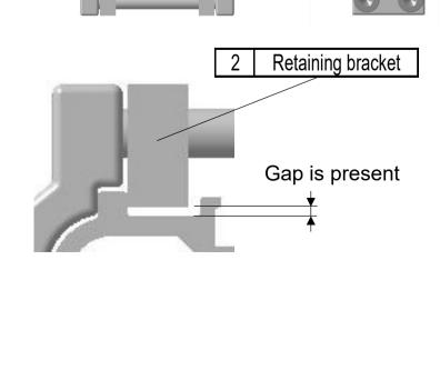
Ideally, the retaining bracket and cylinder tube should remain parallel so that holding force is distributed evenly.
