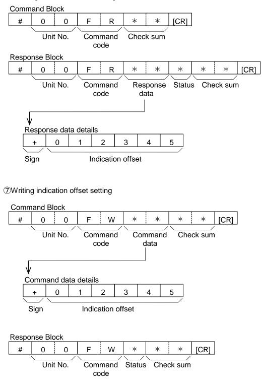
8 Reading cylinder stop output setting
