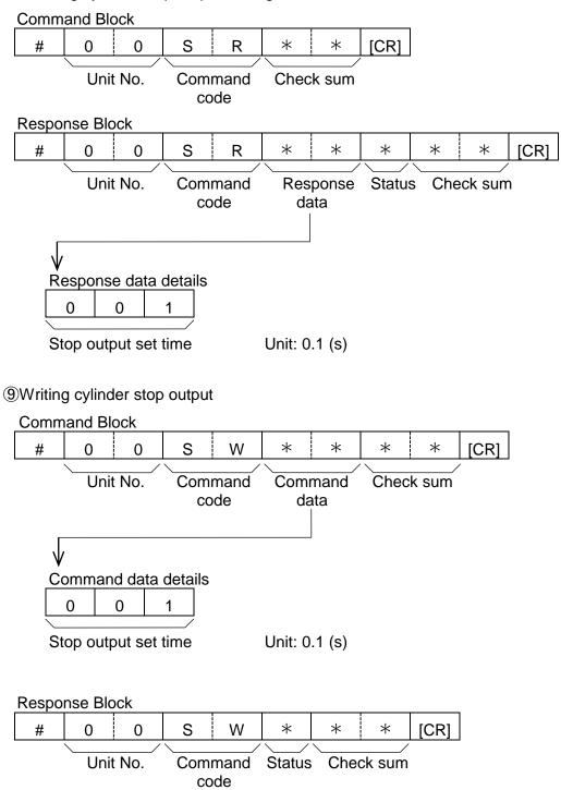
Note: Setting time for cylinder stop output is 1 (0.1 second) or more. For zero (0), error occurs.
