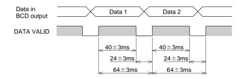
When readout enable signal is ON (when output transistor is ON), data will be valid. BCD output is continuously transmitted in the timing as shown above.
