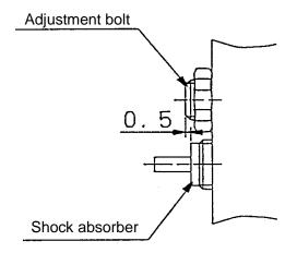
② When shock absorber is used in the range of air cushion stroke, air cushion needle shall be almost full opened (about one and a half turn from the position of full close.)
