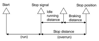
When cylinder is stopped intermediately, "idle running distance" (from detection of stop signal to beginning of brake operation) and "braking distance "(from beginning of brake operation to slider stop) are occurred as shown in the figure left.
