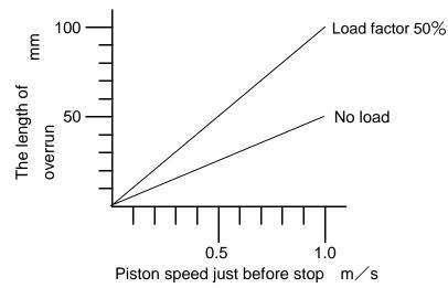
Operating pressure 0.5MPa Brake releasing pressure 0.3MPa Mounting position Horizontal
