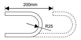
Reciprocating with bending speed 100times/min.
