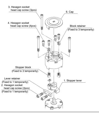
Be careful with the notes on the right drawing for mounting the stopper lever and lever holder.
