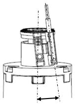
Not parallel to the center of the product (Not the correct position - Re assemble)
