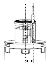
Parallel to the center of the product (recommended condition for mounting)
