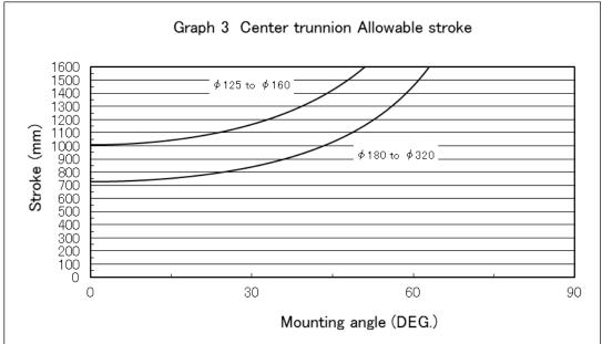
4) The relation between cylinder size and max. stroke by the mounting style Table 2 shows max. usable stroke found by calculation on the assumption that the force generated by cylinder itself acts on piston rod or piston rod and tube as buckling force.
