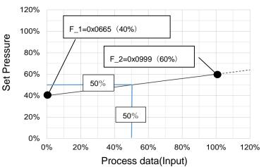
The set pressure output 50% when the process date input 50%
