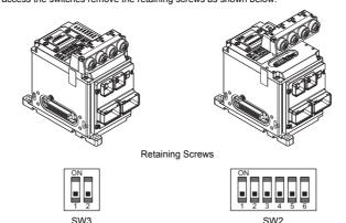
When the DIP-Switches have been set ensure the M12 connector block and all retaining screws are refitted. (torque = 0.4 Nm) The module must be in a fully assembled state with all parts securely fastened before using the product.
