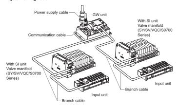
The EX500 range of units can be connected to open fieldbus to realize the reduction of input or output device wiring and the distributed control system.
