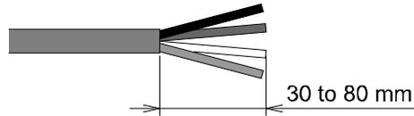
2, Removal of sheath of signal cable
