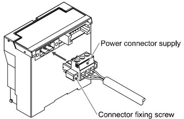
Applicable cable of the power supply connector
