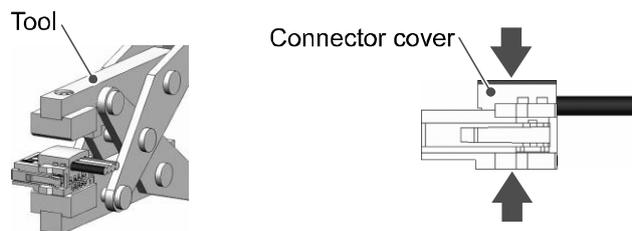
(2) Squeeze firmly on the DWT-A01 Pliers until the lock on the connector clicks into place.
