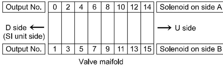
\*: Standard wiring of the manifold is for double-solenoid valves and the output number starts at the A side and then B side in that order as shown in the figure a.
