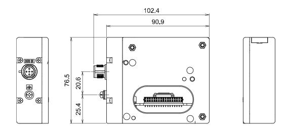
•If a fieldwireable connector is used for the power supply connection, and the SI unit is installed directly to a solenoid valve manifold, the connector should be  $\phi$ 16 mm or less. If the connector is a larger diameter it will interfere with the clamping face.
