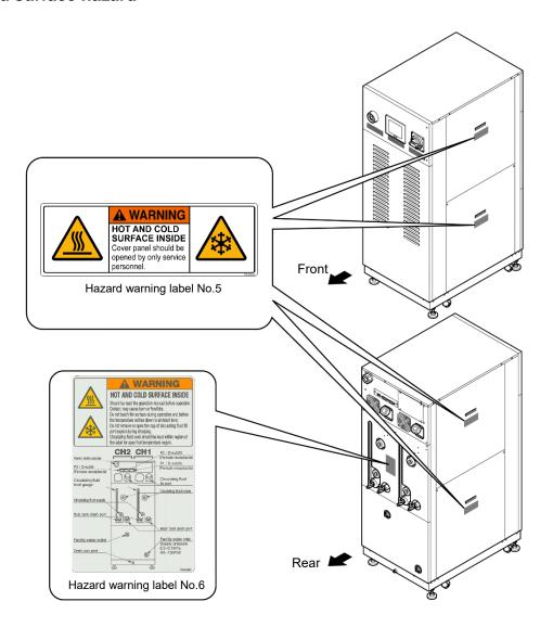
Figure 1-8 Hot/Cold Surface Hazard
