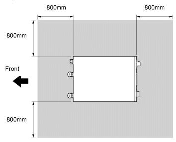
Figure 3-2 Recommended Installation Location
