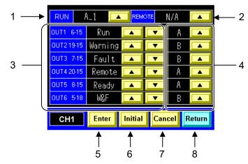
Figure 5-47 "CH1(2)DIO Communication Setting Screen 2"
