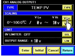
Figure 5-67 "CH1(2) Analog Output Setting Screen 1, 2"
