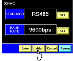
Figure 5-44 "Serial Communication Setting Screen 2"
