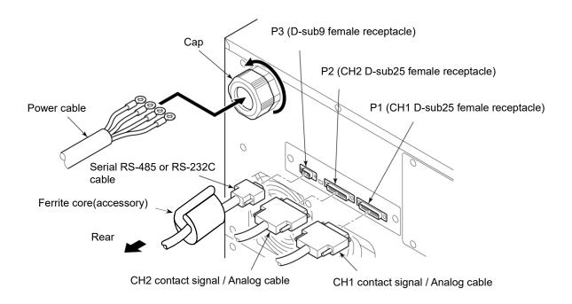
Figure 3-8 Power Cable Insertion and Communication Cable Connection
