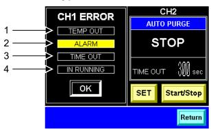
Figure 5-83 "Purge Mode Screen": ERROR Window (E.g.: ALARM)
