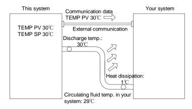
Figure 8-3 Example of Offset Function
