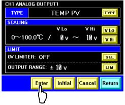
Figure 5-65 "CH1(2) Analog Output Setting Screen 1, 2"
