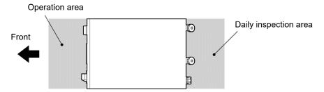
Figure 3-3 Installation Location
