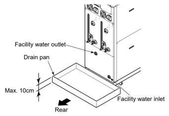
Figure 7-3 Drain Pan Attachment
