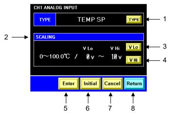
Figure 5-53 "CH1(2) Analog Input Setting Screen 1"
