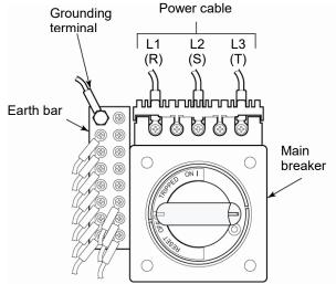
Figure 3-9 Connection of Power Cable and Grounding Terminal
