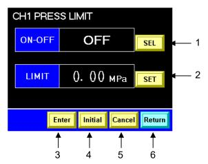
Figure 5-78 "Circulating Fluid Discharge Pressure Limit Setting Screen"
