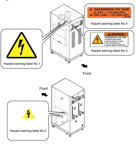
Figure 1-7 High Voltage Hazard
