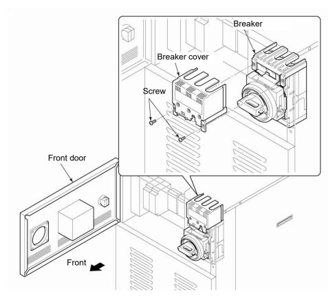
Figure 3-7 Removal of Breaker Cover
