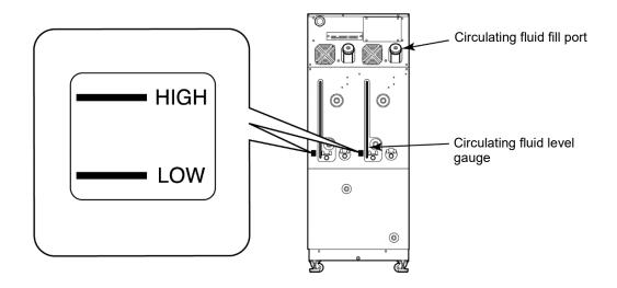
Figure 4-1 Circulating Fluid Filll Port and Circulating Fluid Level Gauge
