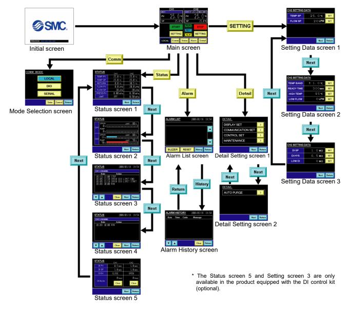
Figure 5-2 Flow Chart of Operation Screen (1)
