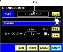
Figure 5-54 "CH1(2) Analog Input Setting Screen 1"
