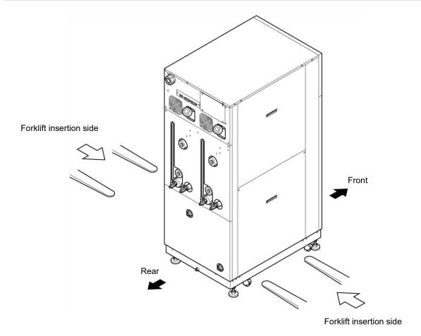
Figure 3-1 Transport with Forklift
