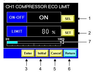
Figure 5-75 "Compressor ECO Limit Setting Screen"
