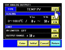
Figure 5-64 "CH1(2) Analog Output Setting Screen 1, 2"
