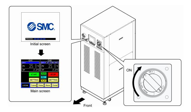
Figure 4-2 Main Breaker at 'ON'
