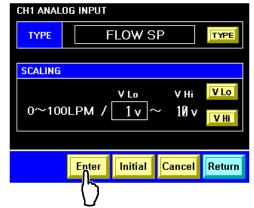
Figure 5-59 "CH1 Analog Input Setting Screen 1"
