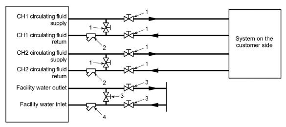
Figure 3-11 Recommended Piping Installation
