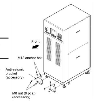
Figure 3-4 Anti-seismic Bracket Attachment
