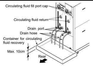
Figure 7-1 Container for Circulating Fluid Recovery
