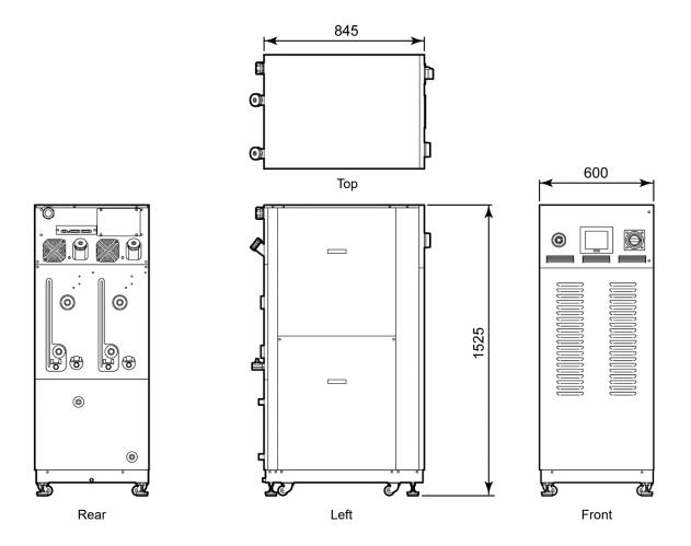
Figure 8-1 Outer Dimensions (Dimensional Tolerance: ±10mm)
