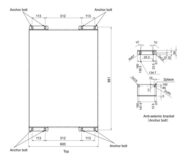
Figure 8-8 Anchor Bolt Mounting Position
