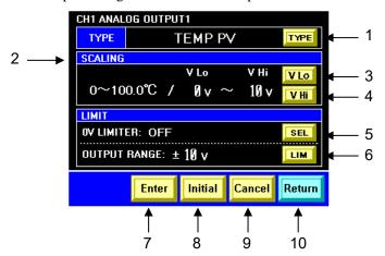
Figure 5-63 "CH1(2) Analog Output Setting Screen 1, 2"
