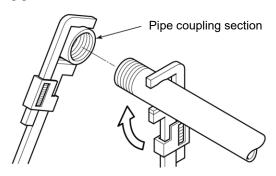
Figure 3-10 Pipe Tightening
