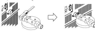
Loosen the M5 screws at the back of the thermo-chiller panel. Mount the particle filter bracket (3). Using tapping screws (8), mount the particle filter bracket to the
