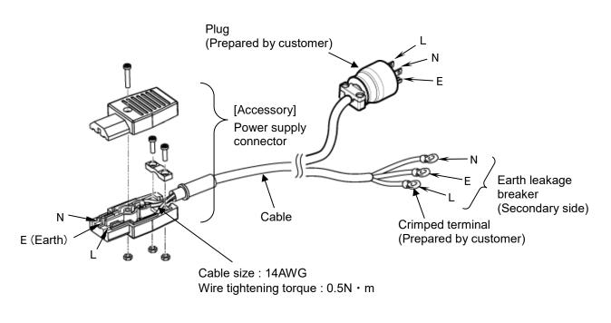
Fig. 3-5 Power supply cable
