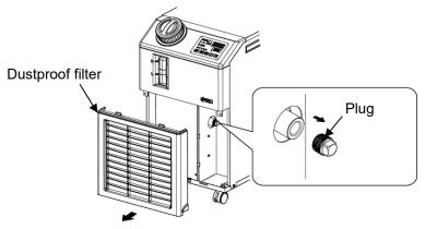
Fig. 8-5 Removal of the plug
