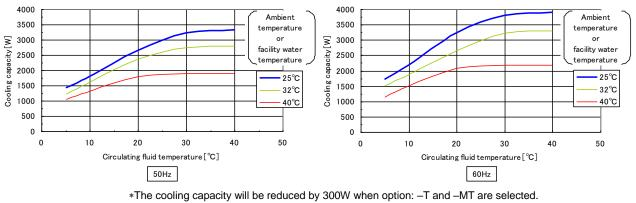
Fig. 9-4 Cooling capacity(HRS030-\*\*-20-(BJMT))
