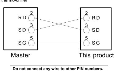
Fig. 3-10 Connection of RS-232C
