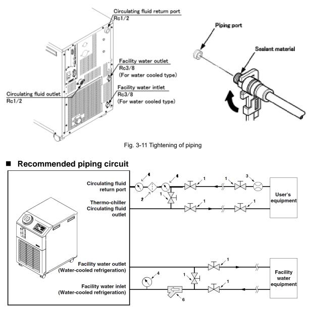
Fig. 3-12 Recommended piping circuit
