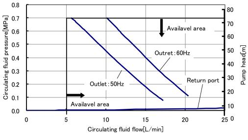
Fig. 9-8 Pump capacity(HRS030-\*\*-20-T)
