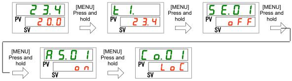
2. Select communication mode from the table below with [▲] key or [▼] key, and confirm by pressing "SEL".
