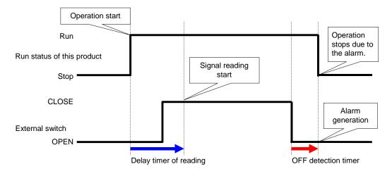
Fig 3-15 Timing chart of external switch monitoring
