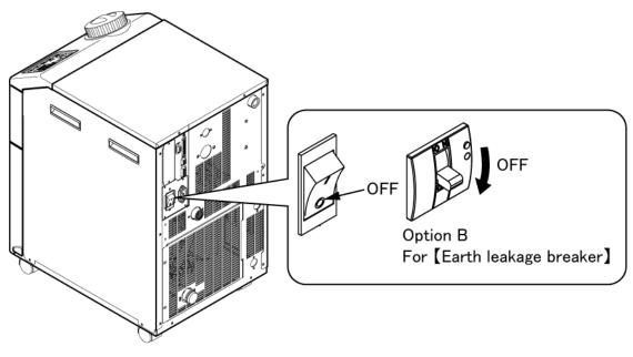
Fig. 1-4 Location of the switch for the power supply
