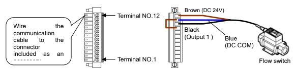
Fig 3-17 Wire the communication cable to the connector included as an accessory.
