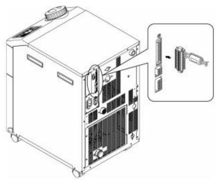
Fig 3-18 Connecting the connector
