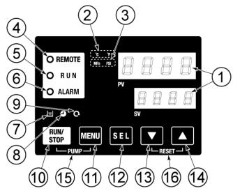
Fig. 2-3 Operation display panel
