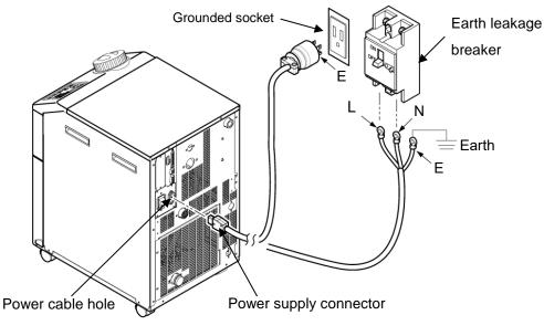
Fig. 3-6 Wiring of power supply
