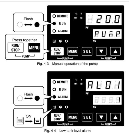
**2.** Press the [RESET] key ( $[\mathbf{V}]$  and  $[\mathbf{A}]$  keys simultaneously) to stop the alarm buzzer.
