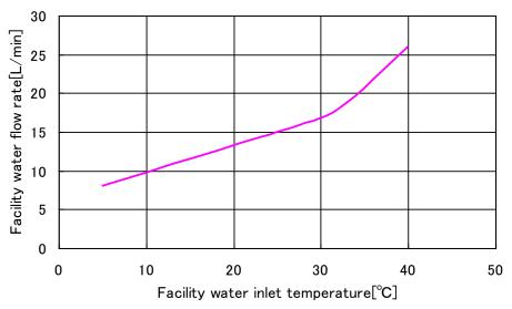
\*The amount of the facility water for the operation with rated circulating fluid, cooling capacity which is described in fig.9-4-1.
