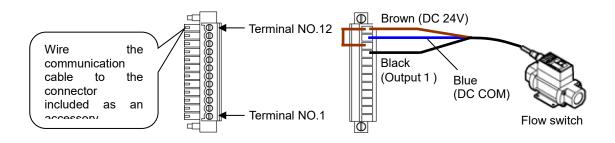
Fig 3-16 Wiring of the external switch (NPN open collector output) (example)
