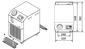
Fig. 3-4 Anti-seismic brackets installing \*4 (four) M8 foundation bolts should be prepared by the customer.
