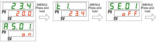
Low tank level Setting and checking
