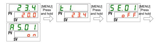
Alarm buzzer sound Setting and checking
