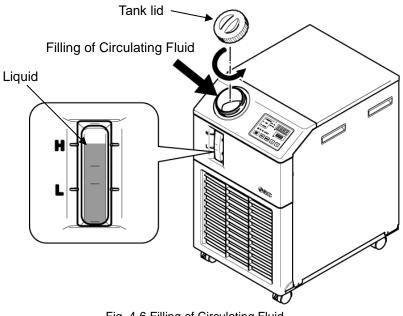
Fig. 4-6 Filling of Circulating Fluid
