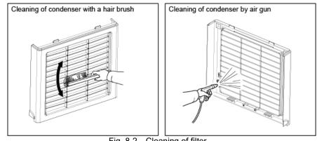
Fig. 8-2 Cleaning of filter
