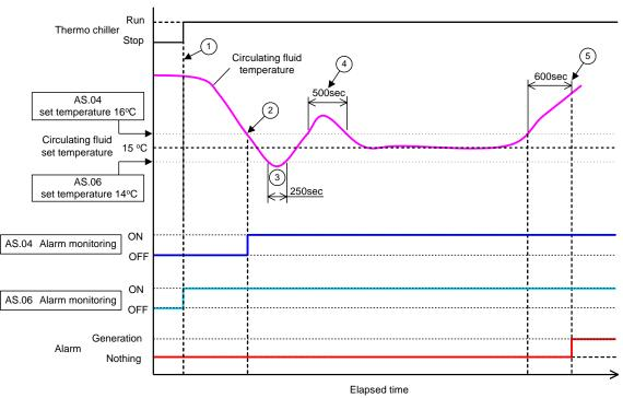
Fig 5.16-1 Alarm generation timing
