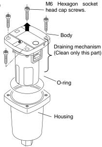
Fig. 2 Disassembly
