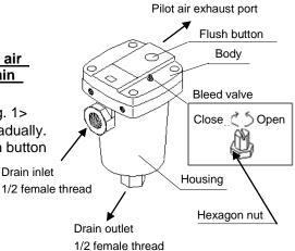
Fig.1 Name and Function of Parts
