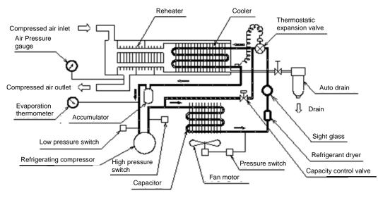
IDF240D Compressed Air and refrigerant circuits
