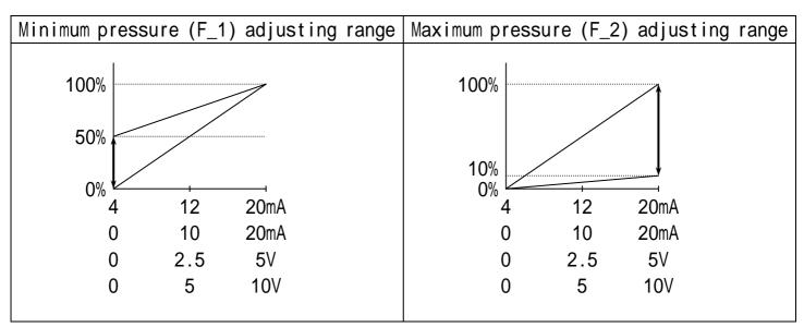
(Note 1): F\_1 is adjustable in a range from 0 to 50% of the rated value.
