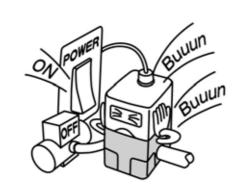
If supply pressure to this product is interrupted or shut off, while the power is still on, the internal solenoid valve will continue to operate and a humming noise may be generated. Since the life of the product may be shortened, shut off the power supply also when supply pressure is interrupted or shut off.
