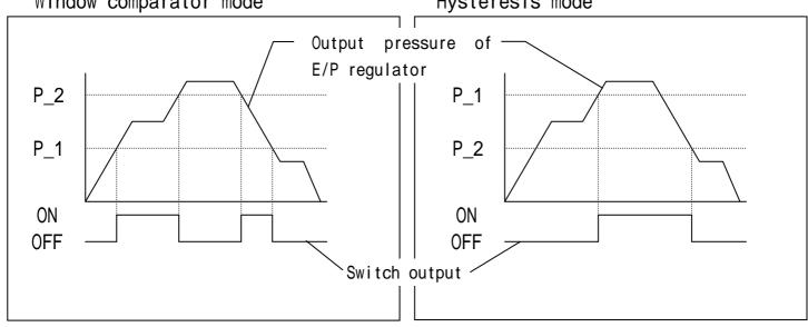
$P_1 = P_2 = 0$ : Out of range mode (The switch output turns on when set pressure is achieved.)
