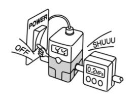
If power to this product is cut off due to a power failure, etc. when it is in a controlled state, residual pressure will be retained temporarily. Handle carefully when operating with output pressure released to the atmosphere, as air will continue to flow out.
