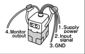
The optional cable connector is a 4 wire type. When the monitor output (analogue output or switch output) is not being used, prevent it from touching the other wires as a malfunction could occur.
