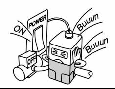
If supply pressure to this product is interrupted or shut off, while the power is still on, the internal solenoid valve will continue to operate and a humming noise will be generated.
