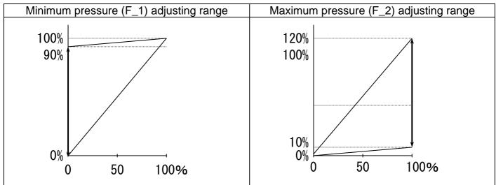
(Note 1): F\_1 is adjustable in a range from 0% to 90% of the rated value. (DEFAULT VALUE: 0%)
