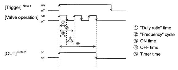
Example 2) Trigger continuous input mode: the trigger starts and stops the valve operation.
