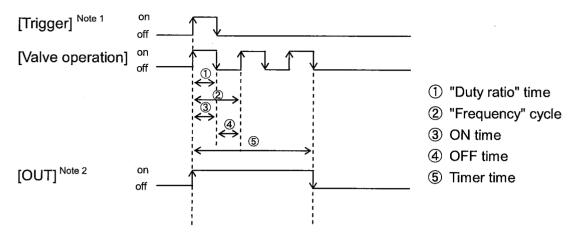
Example 4) Trigger one shot input mode: the trigger starts and stops the valve operation.
