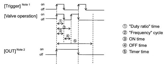
Note1: Trigger turns ON when terminal No.8 is connected to GND.
