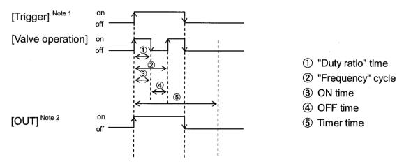
Example 3) Trigger one shot input mode: the trigger starts, and the timer stops, the valve operation.
