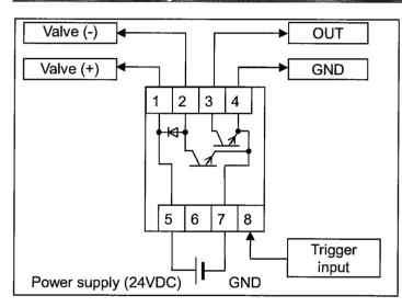
Valve specification: 24 VDC 4 W or less
