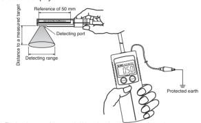
\*: The detecting range of the sensor is 180 mm (at a detection nce of 50 mm)
