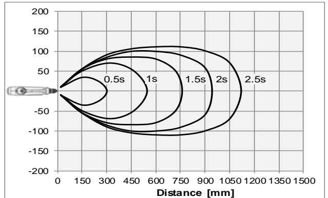
2) Supply pressure 0.1 MPa Consumed flow rate 119 L/min (ANR)
