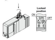
Carefully check the manual override projection amount. Max. (at OFF): 3.7 mm
