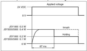
Since the voltage will drop by approx. 0.5 V due to the transistor, pay attention to the allowable voltage fluctuation. (For details, refer to the solenoid specifications of each type of valve.)
