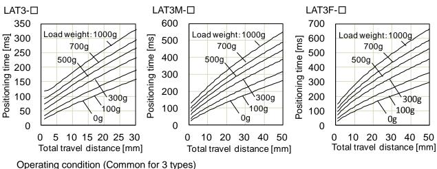
Mounting orientation: Horizontal / vertical Step data input method: Takt input method (Triangle wave operation)
