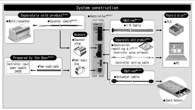
Note 1) "Options" such as controller and cables can be added to the How to Order for the main products (Card Motor and Card Motor controller). Refer to How to Order for details.
