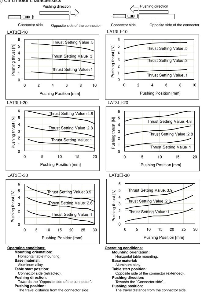
Fig. 4-1 Thrust force characteristics (guideline).
