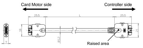
Note) The actuator cable is direction dependent. Connect the Card Motor side of the cable to the Card motor, and vice versa. A small area of the connector is raised on the controller side.
