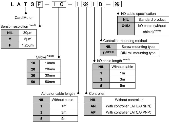
Note1) Refer to the table below for the Card motor model resolution and stroke available.
