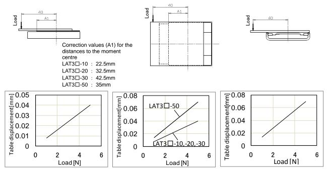
Fig4-5 Table displacement (guideline)
