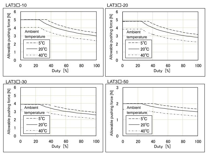
Fig. 4-3 Allowable thrust force setting values.
