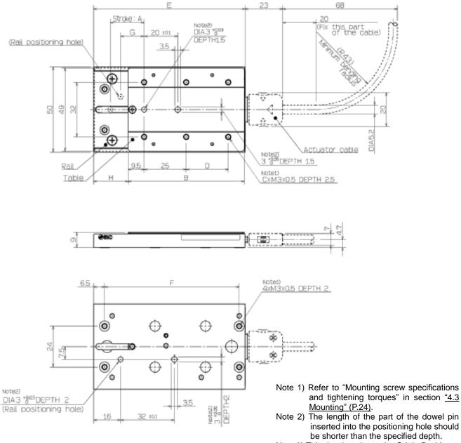
be shorter than the specified depth. Note 3) This drawing shows the Origin Position. Note 4) The G and H Origin position dimensions are reference values (guidelines).
