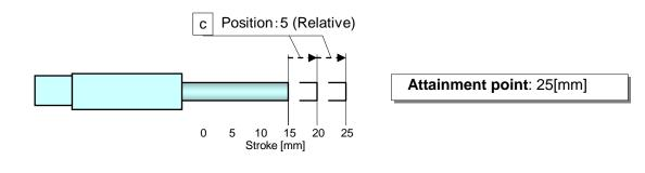
Condition 2) 15mm position  $\rightarrow$  **Step no.1**  $\rightarrow$  **Step no.1** (Move M: Relative)
