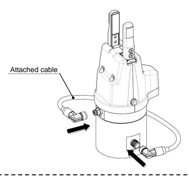
(4)For mounting attachment For mounting and removal of the attachment, refer to the drawing below. Refer to P16, "5-2 Installation" for mounting of the finger to the attachment.
