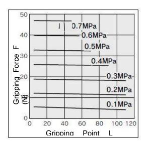
Internal gripping state Indication of effective gripping force
