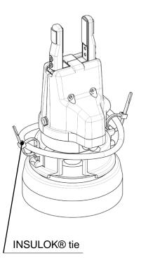
$^{\ast}$  Use a cross recessed resin round head screw (M4 x 6) as a plug when the INSULOK® cable tie is not used.
