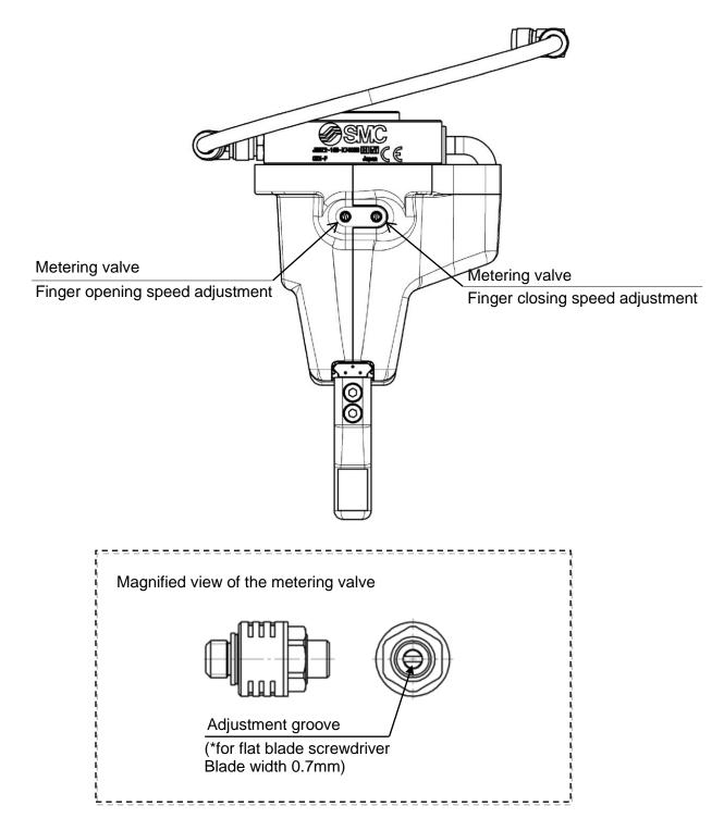
\* Use a flat blade screwdriver for adjusting the restriction of the metering valves.
