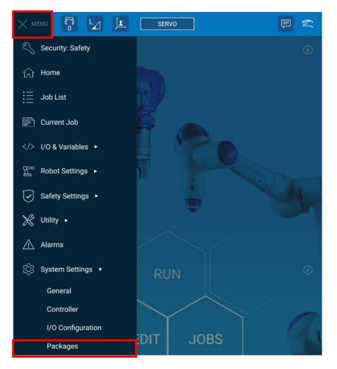
3. Open the "Packages" tab and tap [+INSTALL] at the upper part of the screen. A pop-up dialog box showing the installable packages will appear. From the package list, select "SMC Air Gripper" and install it.
