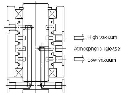
Using atmospheric release port
