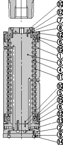
Component Parts/(MQR1 - M5, 1 circuit)
