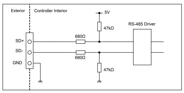
Note 1) There is no terminal resistor built into the controller communication circuit.
