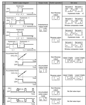
\*1: In window comparator mode, the hysteresis is fixed at 3 digits. When setting, allow 7 digits or more between Set point 1 and Set point 2.
