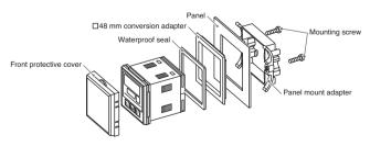
Removing the panel mount adapter The product with panel mount adapter can be removed from the installation by removing 2 screws and releasing the hooks at the sides. The hooks can be released by inserting a suitable thin card.
