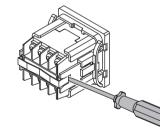
•Lever the hook to the outside to remove the adapter (See below). •If the panel mount adapter is pulled with the hook engaged, the product or the panel mount adapter will be damaged.
