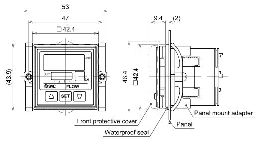
PF2 $\square$ 20 $\square$  + panel mount adapter (ZS-26-B) + front protective cover (ZS-26-01) +  $\square$ 48 mm conversion adapter (ZS-26-D)
