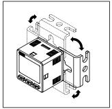
\*Bracket can be mounted on 4 sides.
