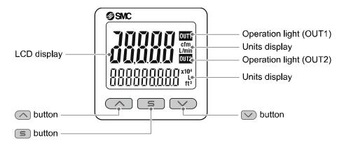
Operation light: Displays the switch operating condition.
