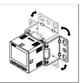
\*Bracket can be mounted on 4 sides.
