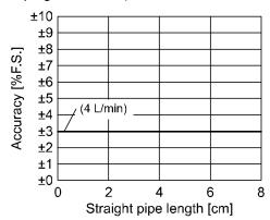
Flow range: 2 to 16 L/min (symbol 20) Pressure: 0.3 MPa
