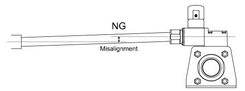
•When a flexible hose is used for the piping, the hose must be fixed with a bracket etc. If it is not fixed, the load weight of the flexible hose and the fluid will be applied to the product.
