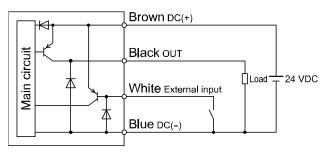
Maximum load current: 80 mA Internal voltage drop 2 V max.
