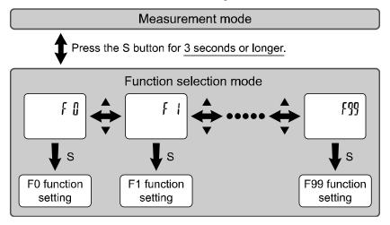
Press the S button for <u>2 seconds or longer</u> to return to measurement mode.
