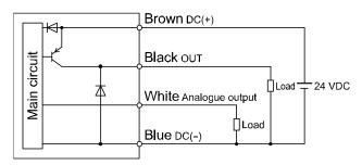
Maximum load current: 80 mA Internal voltage drop 1.5 V max.
