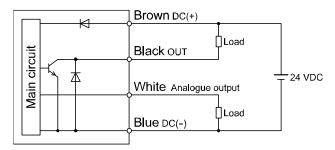
Maximum applied voltage: 28 V Maximum load current: 80 mA Internal voltage drop 1.5 V max.
