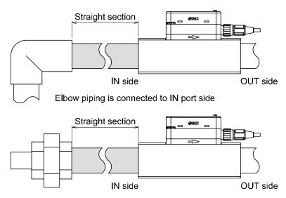
Piping with different diameter is connected to IN port side
