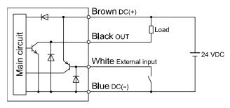
Maximum applied voltage: 28 V Maximum load current: 80 mA Internal voltage drop 1.5 V max.
