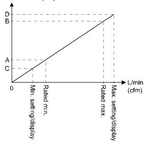
oConversion formula of the process data and flow measurement value
