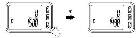
•When ▲ and ▼ buttons are pressed simultaneously for 1 second or more, the set value is displayed as [ - - - ], and the set value will be set to the same as the displayed value automatically (snap shot function) (Refer to page 66). Afterwards, it is possible to adjust the value by pressing ▲ or ▼ button.
