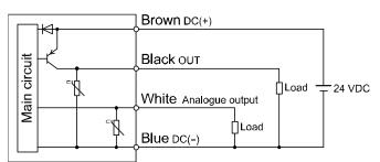
Maximum load current: 80 mA Internal voltage drop 2 V max.
