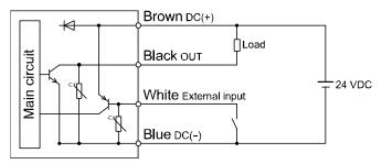
Maximum applied voltage: 28 VDC Maximum load current: 80 mA Internal voltage drop 1 V max.
