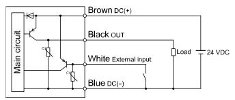
Maximum load current: 80 mA Internal voltage drop 2 V max. External input: Input voltage of 0.4 V max. (reed or solid state input) for 30 ms or longer
