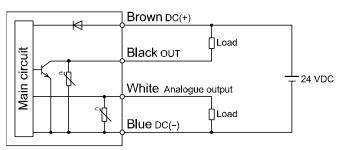
Maximum applied voltage: 28 VDC Maximum load current: 80 mA Internal voltage drop 1 V max. CS: Analogue output: Select 1 to 5 V or 0 to 10 V. Output impedance: 1 k
