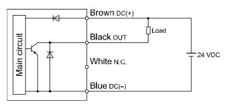
Maximum applied voltage: 30 V Maximum load current: 80 mA Internal voltage drop 1.5 V max.
