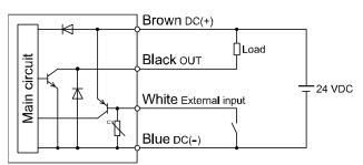
Maximum applied voltage: 30 V Maximum load current: 80 mA Internal voltage drop 1.5 V max. External input: applied voltage of 0.4 V max. (reed or solid state input) for 30 ms or longer
