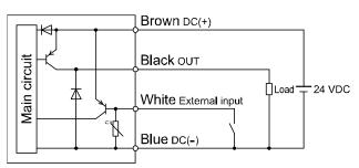
Maximum load current: 80 mA Internal voltage drop 2 V max. External input: Input voltage of 0.4 V max. (reed or solid state input) for 30 ms or longer
