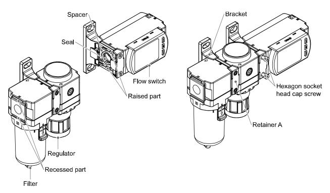
•The following options are required for coupling with modular F, R, and L combinations. They are separately prepared by the user.
