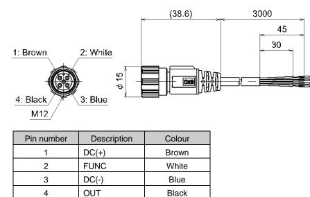
\*: 4-wire lead wire with M12 connector for PF3A series.
