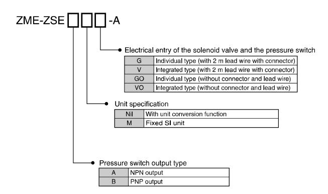
Integrated cable assembly for the solenoid valve/pressure switch
