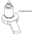
When connecting the pressure sensor, apply a wrench to the
