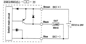
Brown lead: Connect to DC power (+) terminal to operate switch
