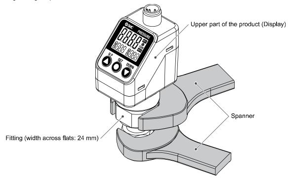
When tightening, do not hold the upper part of the product (Display) with a spanner.
