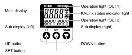
Operation light: Displays the switch operating condition.
