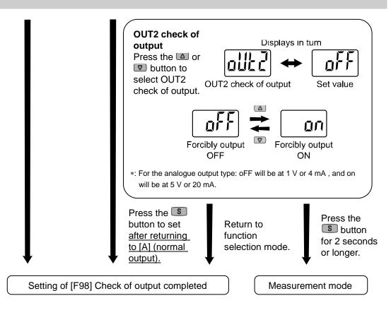
\*: If the S button is pressed for 2 seconds or longer, the mode is returned to measurement mode regardless of the current mode.
