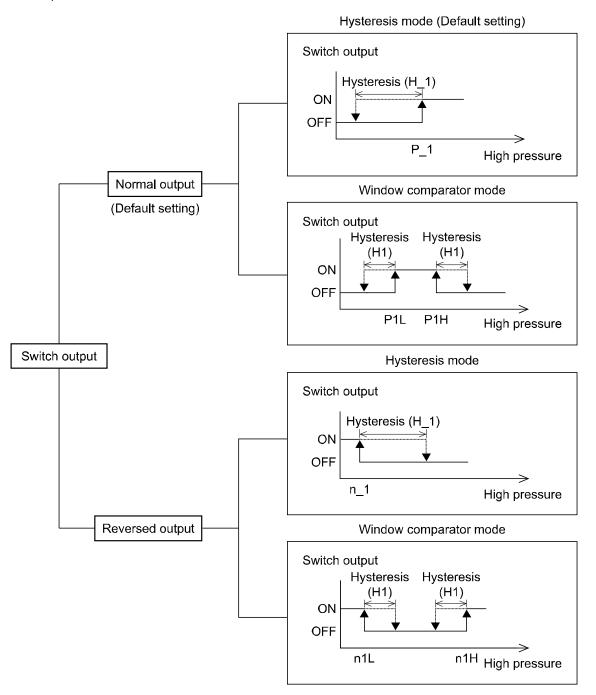
If the set point when the switch output is changed is outside the set pressure range due to switching between normal and reversed output, the hysteresis will automatically be compensated.
