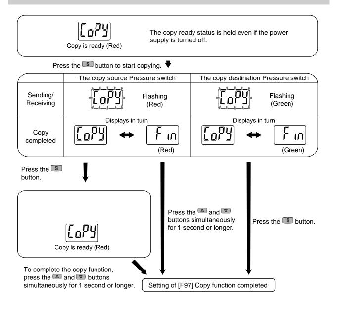
\*: If the copy to the copy destination pressure switch is not completed, it is detected as a copy function sending/receiving error. Press the and v buttons simultaneously for 1 second or longer to return to measurement mode. Then, check the wiring and specifications of the switch and retry the copy function.
