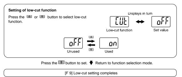
\*: Measurement mode can be returned from any setting items by pressing and holding the S button for 2 seconds or longer.
