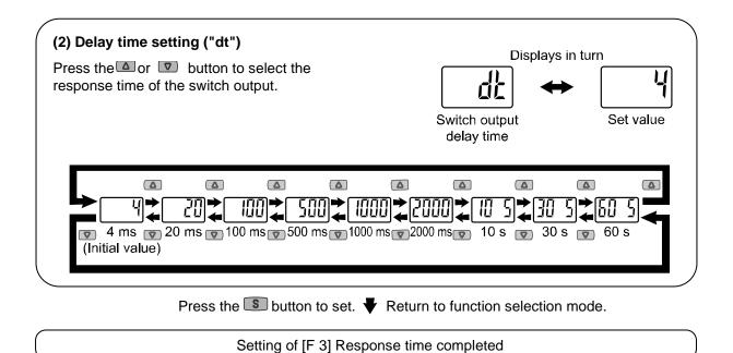
\*: Measurement mode can be returned from any setting item by pressing the S button for 2 seconds or longer.
