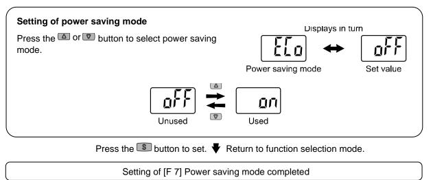
In power saving mode, any key operation will return the normal display. If there is no key operation for 30 seconds, the display will return to power saving mode (only in measurement mode).
