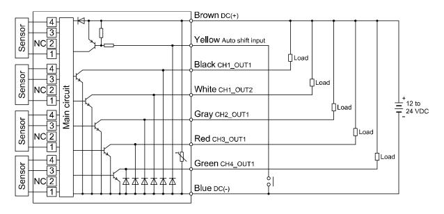
PSE201A-(M)□: PNP open collector 5 outputs + Auto-shift 1 input
