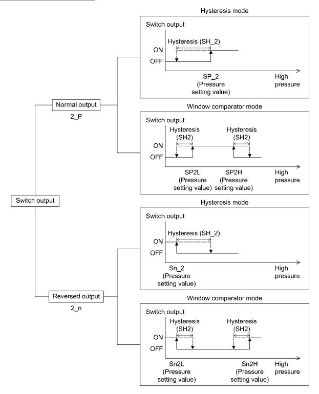
If the set value when the switch output is changed is outside the set pressure range due to switching between normal and reversed output, the hysteresis will automatically be compensated.
