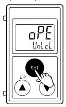
(2) Select the key-locking/un-locking with UP or DOWN button, and press the SET button to set.
