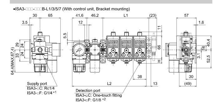
\*: Only bracket mounting is applicable for use with a control unit.
