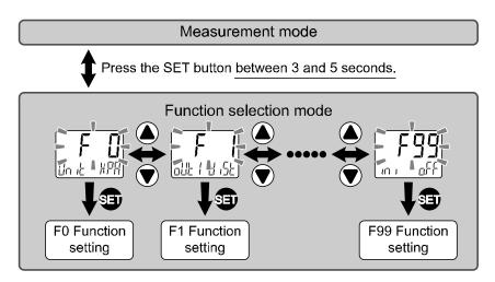
\*: Some products do not have all the functions. If no function is available or selected due to configuration of other functions, [- - -] is displayed on the sub display (right).
