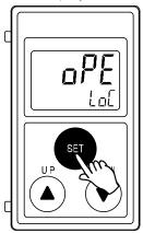
(2) Select the un-locking [UnLoC] with UP or DOWN button. Setting is recognized by pressing the SET button, then security code is required.
