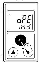
(2) Select the key [LoC] with UP or DOWN button, and press the SET button to set.
