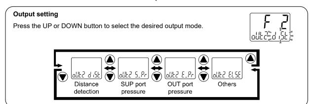
Press the SET button to set. Move on to output mode setting.
