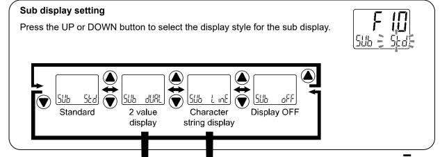
[dUAL] 2 value display is selected Press the SET button to move on to sub display (left) setting. [LinE] Character string display is selected
