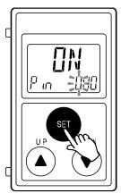
(4) If inputted security code is correct, the indication of the main display changes to [UnLoC], and pressing the one of UP, SET or DOWN button releases key-lock and the measurement mode returns. If the security code entered is incorrect, [FAL] will be displayed, and the security code must be entered again. If the wrong security code is entered 3 times, [LoC] is displayed and the device returns to measurement mode.
