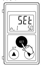
(2) Change the set value with the UP or DOWN button, and press the SET button to set the value. Then, the setting moves to hysteresis setting. (The snap shot function can be used. (Refer to page 84))
