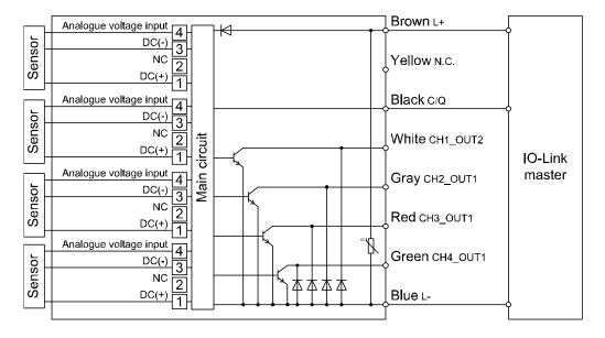
•When used as a switch output device
