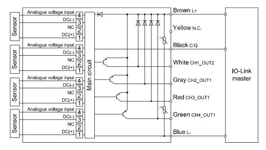
•When used as a switch output device
