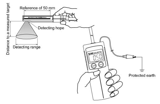
\*: The detecting range of the sensor is 180 mm (at the best measurement distance of 50 mm).
