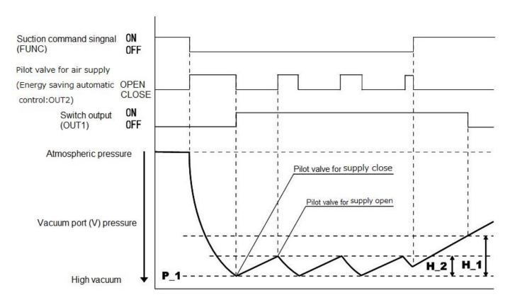
See below for the energy saving control operation and the set values which are preset to the switch. If the operation shown below is acceptable, then keep these settings.
