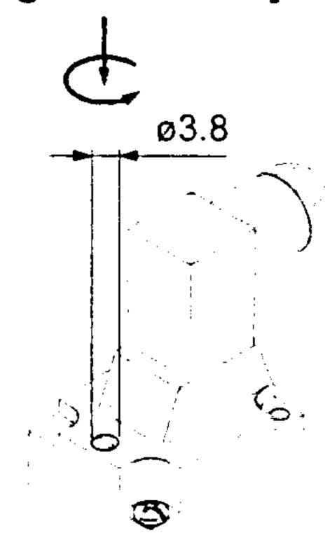
Push the manual override button with a small screw driver until it stops. Turn it in the counter-clockwise direction at 90°, and it is locked. Turn it right to release.
