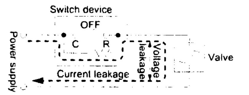
AC coil: 10% or less rated voltage
