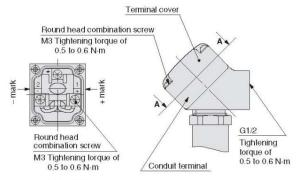
View A-A (Internal connection diagram)
