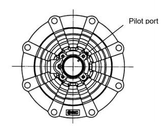
Fig. Pilot port position for pilot valve
