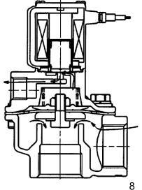
The pressure in the pressure chamber reduces by exhausting air to the pilot exhaust.
