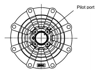
Fig. Pilot port position for pilot valve
