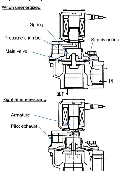
The fluid enters the IN side and goes through the supply orifice to fill the pressure chamber.
