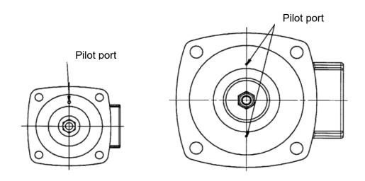
Fig. Pilot port posion of the diaphragm assembly
