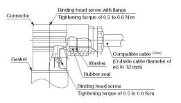
Note) If using a cable with ouside diameter of  $\Phi 9$  to 12mm, remove the internal part of the rubber seal before using.
