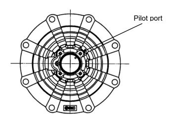
Fig. Pilot port position for pilot valve
