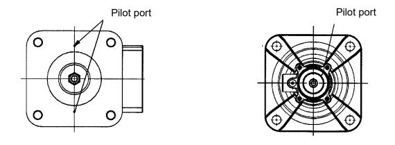
Fig. Pilot port position for main body
