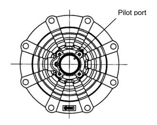
Fig. Pilot port position for pilot valve
