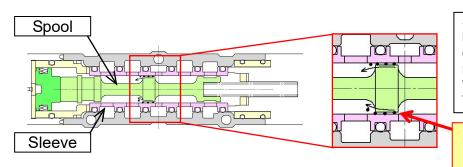
Since the larger main valve leakage increases the cleaning effect while fine particles can pass through, it is difficult for foreign matter to accumulate at the main valve.
