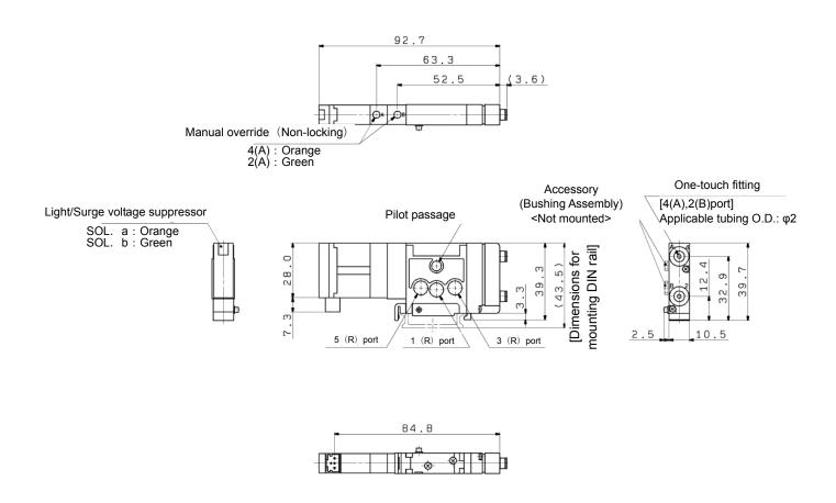
Note: The illustrations show the SZ3260-5LOZ-C2-X84 model. The dimensions other than the A, B port sizes are the same as the standard model.
