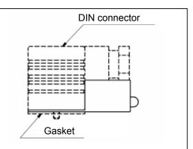
Assemble the spacer with light between the DIN connector and gasket for IP40.
